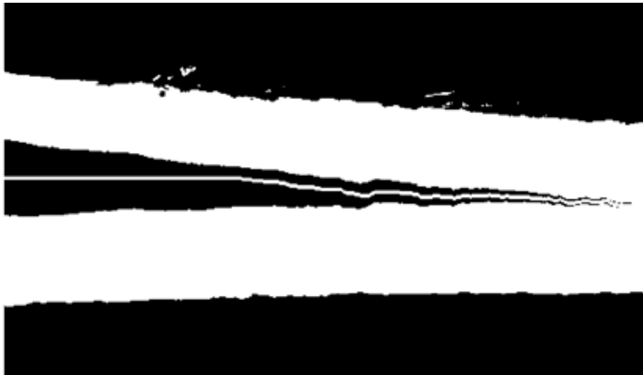
Figure 3.7 Matlab image processing output for a DCB sample (white bands), showing the original opened crack flanks (black wedge) and the trace of the crack tip as it propagates (white central line).
