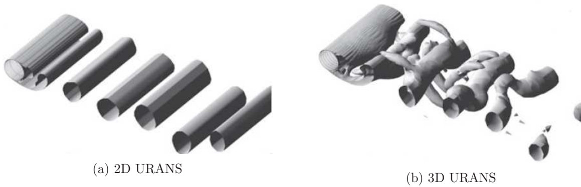
Figure 1.1: Flow over a circular cylinder using the SA-URANS model. Figure reproduced from Spalart (2009).
