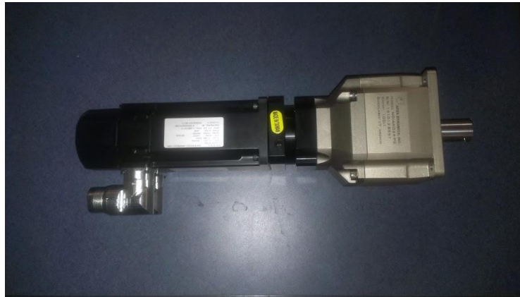
Figure 15. Kollmorgen AKM23C Servomotor with 100:1 gearbox
