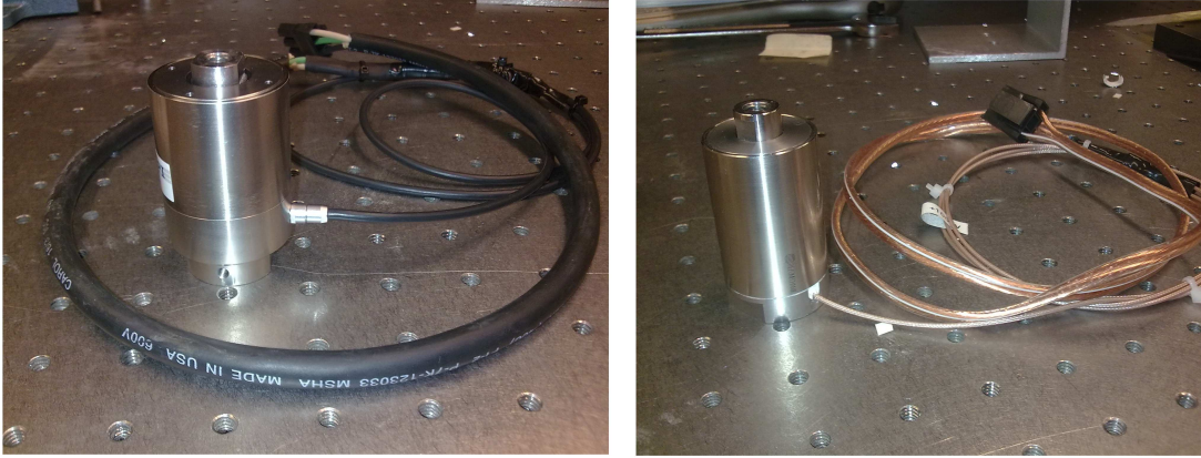
Figure 1.2 Picture showing close up of two of the transducers used for this study. On the left is a Physik Instrumente transducer (PI2533) with stack length 33 mm and stack diameter 25 mm and on the right is a Piezomechanik transducer (PM2540) with stack length 40 mm and stack diameter 25 mm.
