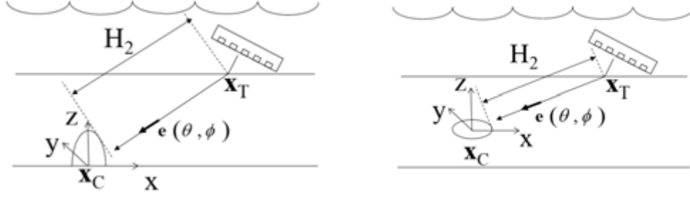
(a) Pulse-echo immersion setup for the EFTOFD sizing of a surface-breaking crack. (b) Pulse-echo immersion setup for the EFTOFD sizing of a volumetric flaw.
