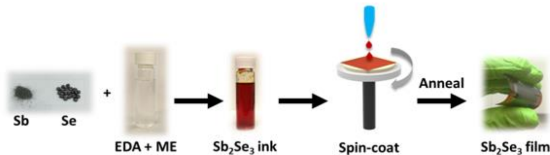
Figure 20. Fabrication scheme for Sb_2Se_3 nanostructure formation on flexible substrates utilizing a molecular ink. The process begins with dissolution of elemental Sb and Se in ethylenediamine (EDA) and 2-mercaptoethanol (ME) to produce a molecular ink that is spin-cast onto a flexible substrate and annealed to form a flexible nanowire-based film.
