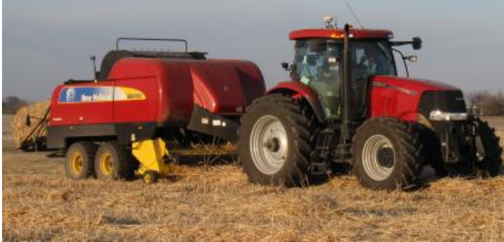
Figure 13: Large square baler used in harvesting trials: Case Puma 210 tractor powering BB9080R large square baler.
