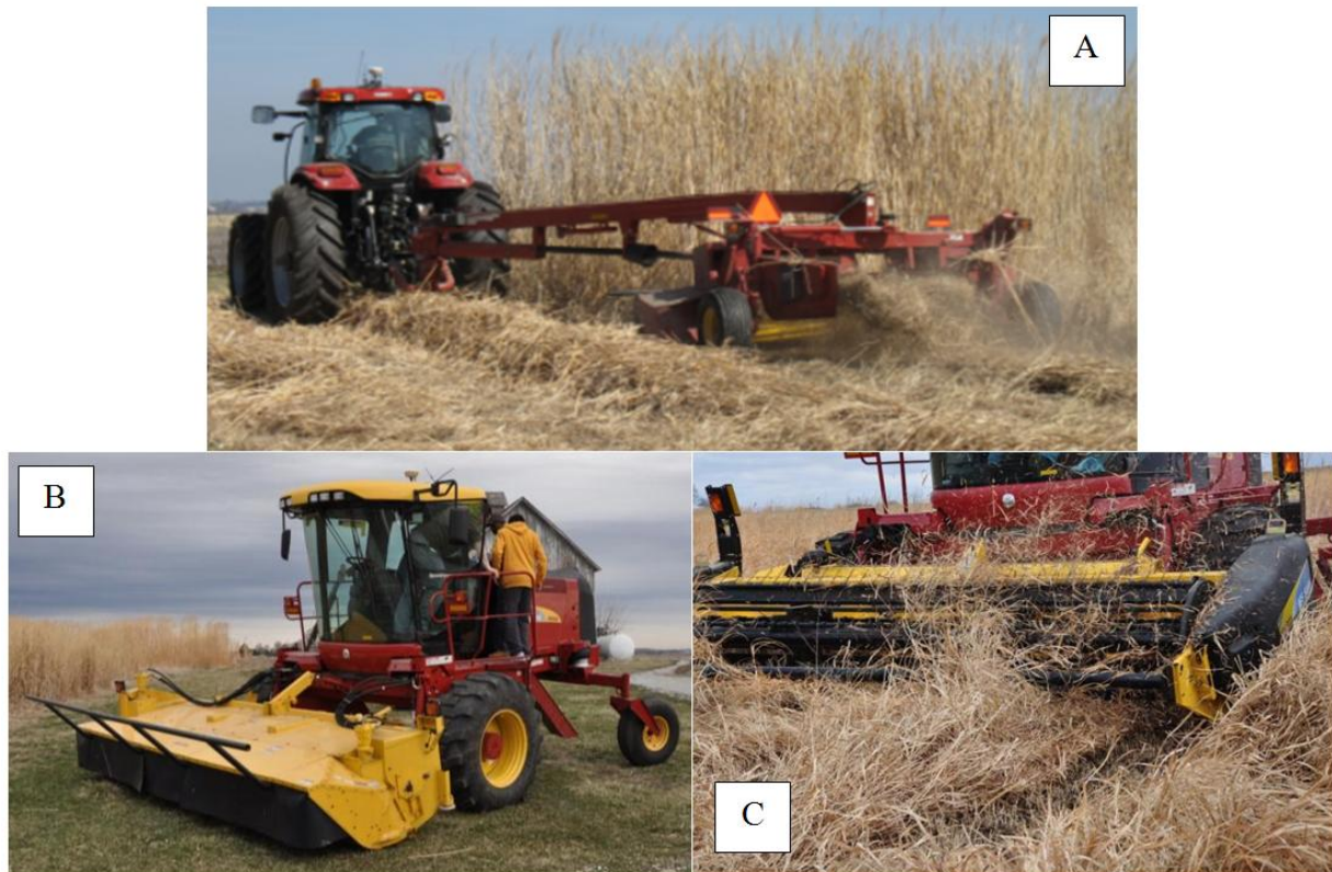
Figure 12: Mowers used in energy crop harvest: Case Puma 210 powering DC 132 rotary disc mower-conditioner (A), self-propelled H8080 with rotary (B), and sickle mower-conditioner heads (C).
