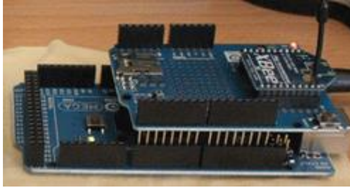
Figure 3.12 Installation of Wireless and SD shield on Mega 2560 with X-Bee transmitter
