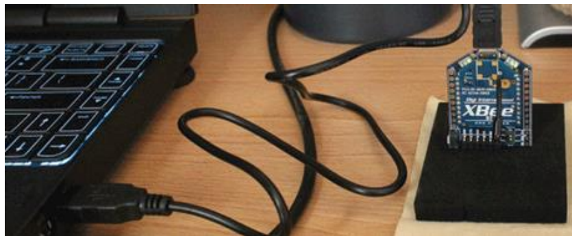
Figure 3.13 X-Bee transmitter connecting with PC through USB shield
