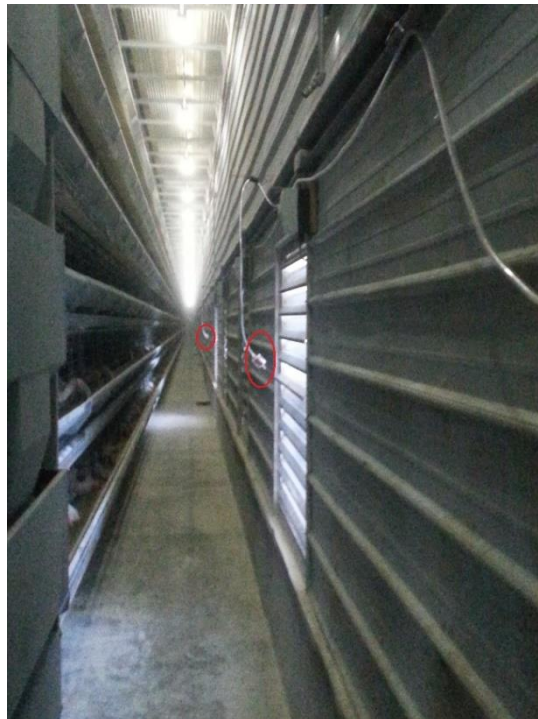
Figure 3.25 Photo of barn air sampling points in first field test
