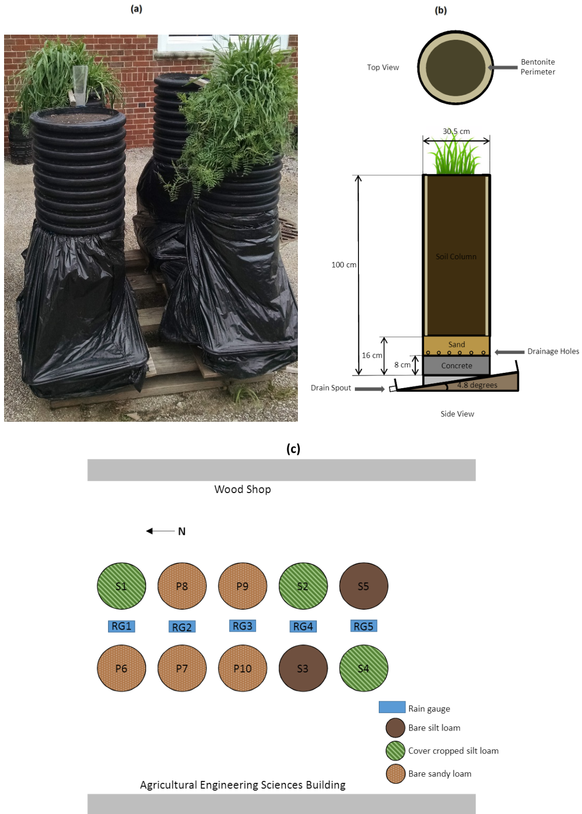
Figure 4.1: (a) Photograph of four silt loam soil columns during the growing season, (b) Scaled drawing of a soil column, and (c) Diagram of outdoor experimental setup including soil columns and rain gauges
