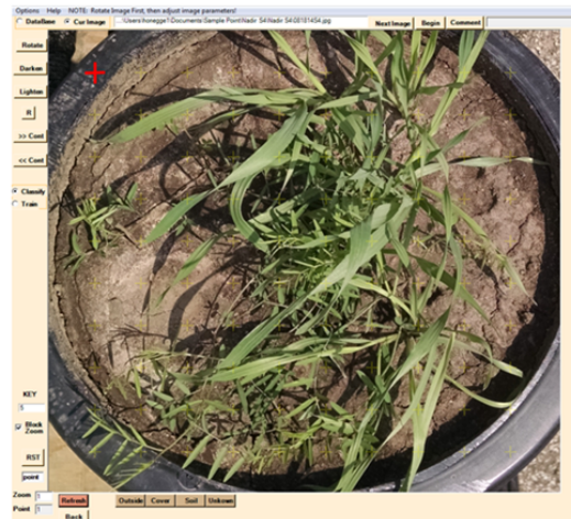
Figure 4.7: SamplePoint software user interface for determining percent canopy cover from orthographic photographs
