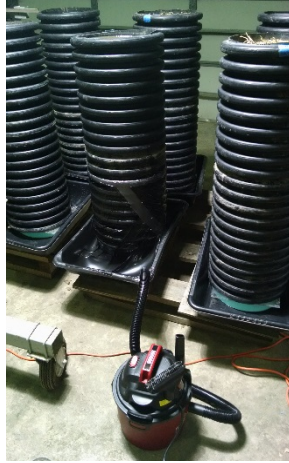
Figure 5.3 Vacuum applying suction at base of bare soil column S3 to force drainage
