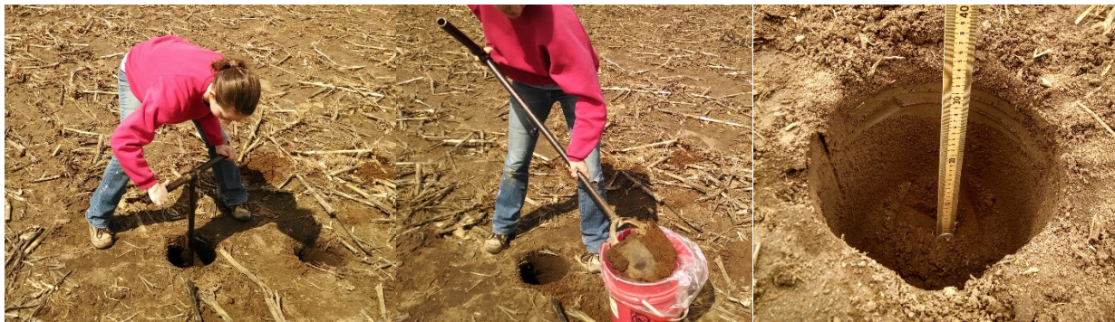
Figure 4.2 Soil collection method using a post-hole auger
