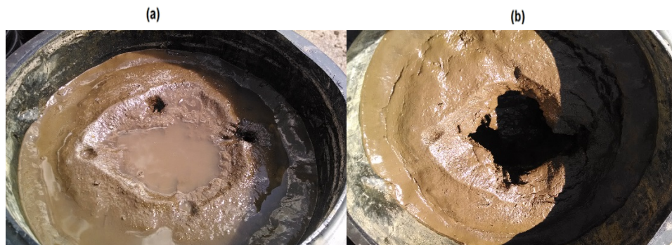
Figure 5.2: (a) Artificial macropore creation in sandy loam columns and (b) Subsequent soil settling
