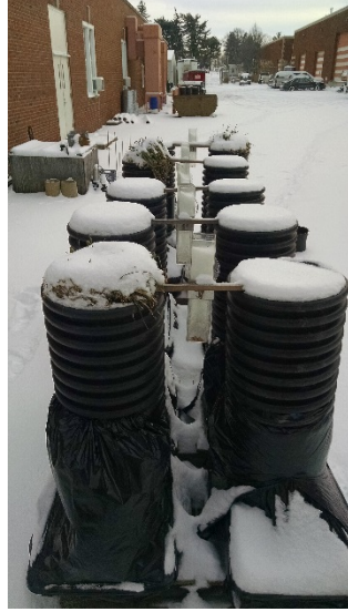
Figure 4.8: Snowfall on outdoor soil columns on 01/06 before spring simulation began
