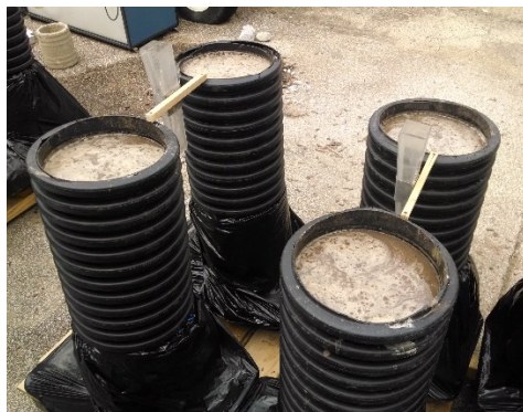
Figure 5.1: Water-logged sandy loam soil columns caused by repacking and lack of soil structure
