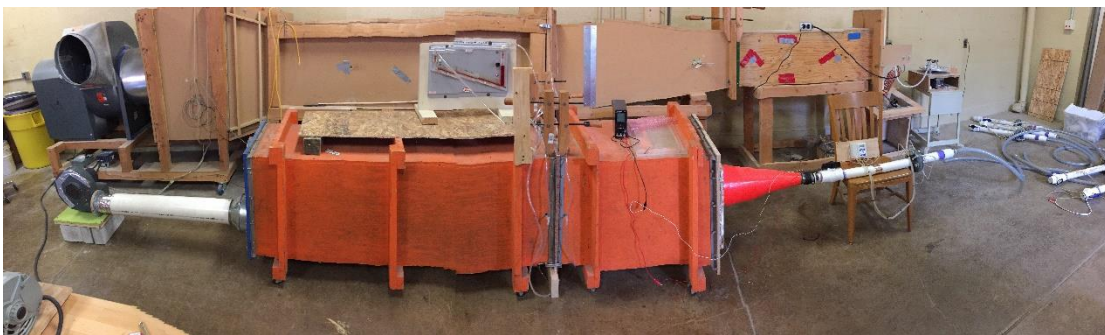
Figure 2.2. The calibration of orifice meters using Chamber-Nozzle Airflow System.
