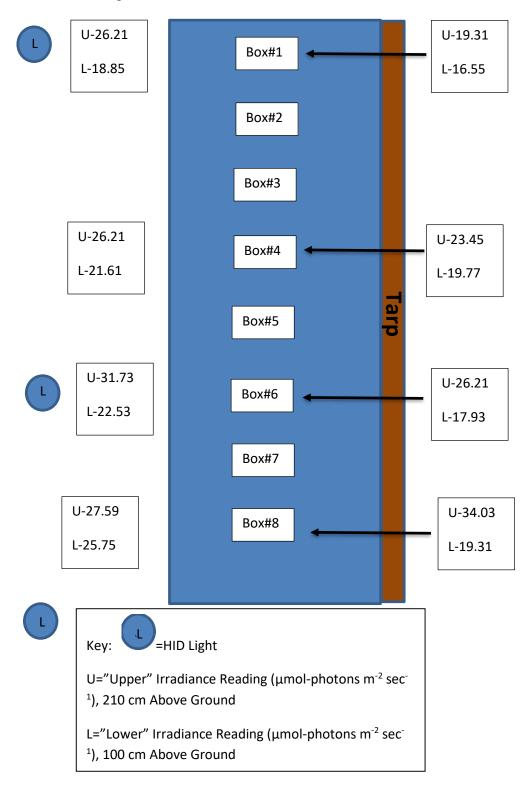
Figure 3-12: Greenhouse Solar Irradiance at 6:13PM CDT
