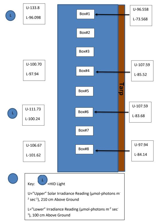
Figure 3-11: Greenhouse Solar Irradiance at 2:30PM CDT
