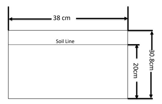
Figure 3-13: Side View of Box Containing Soil and Rice Seeds
