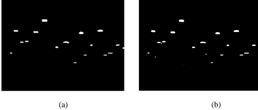
Figure 6.1. The value of T_2 effects the feature detection result. (a) Detected features with T_2 = 50 . (b) Detected features with T_2 = 5 .
