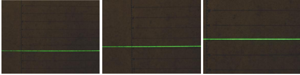
Figure 5.3. The vertical location of the laser mark changes with the distance to the camera. The object is closer to the camera on the right side image.
