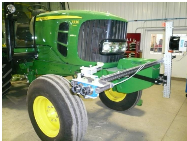
Figure 7.1. The sensor mounted on a tractor by a cross steel frame.
