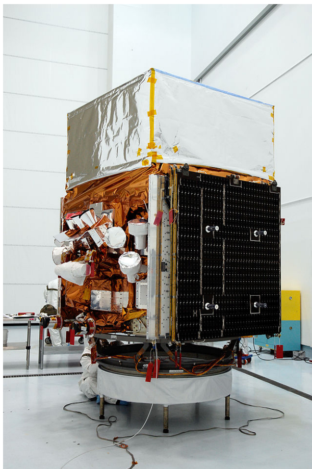
Figure 27: LAT on the payload attach fitting. NASA/ Jim Shiflett.
