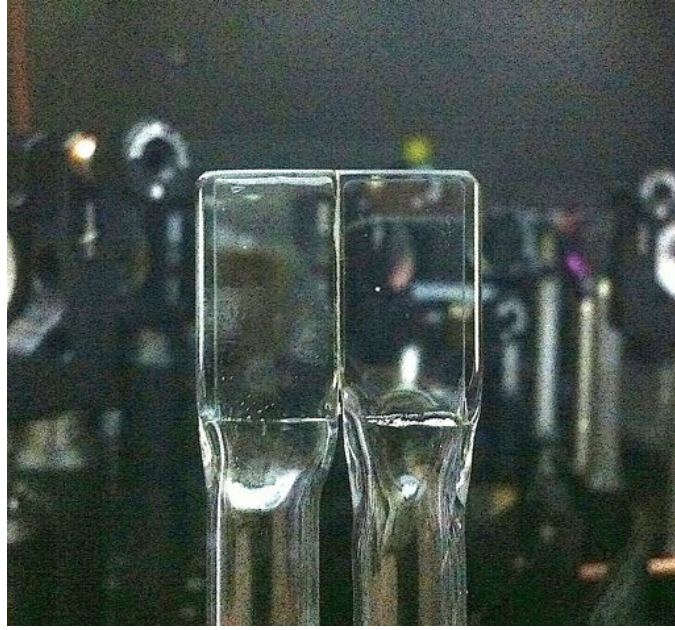
Figure 9.1.: Multi-region 2 mm vapour cell developed in collaboration with the Chemistry Department at Durham University. The separation between the chambers is approximately 800\text{ }\mu\text{m} .
