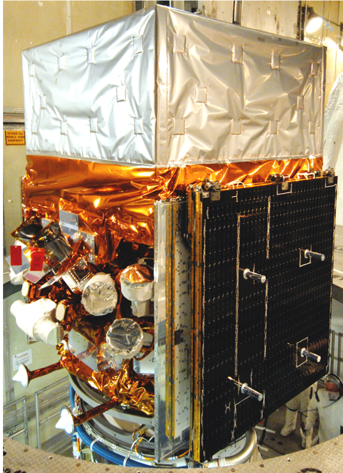
Figure 2.2: The Fermi satellite, shortly before being launched into space. One of the solar panels can be seen folded onto the side of the spacecraft. Image credit: NASA/DOE/ Fermi LAT Collaboration.
