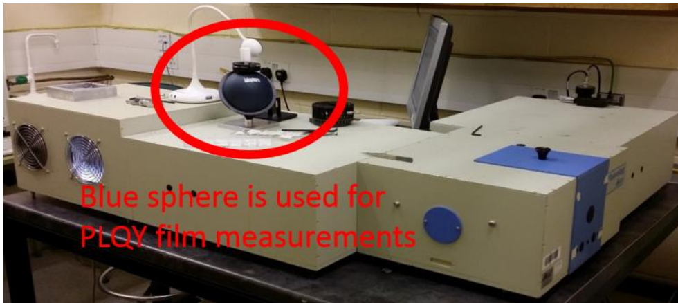
Figure 3.5 Jobin-Yvon Horiba Fluorolog FL3-22 spectrofluorimeter in Durham university OEM research laboratory. The blue sphere on top of the spectrofluorimeter is used for PLQY measurements of films.
