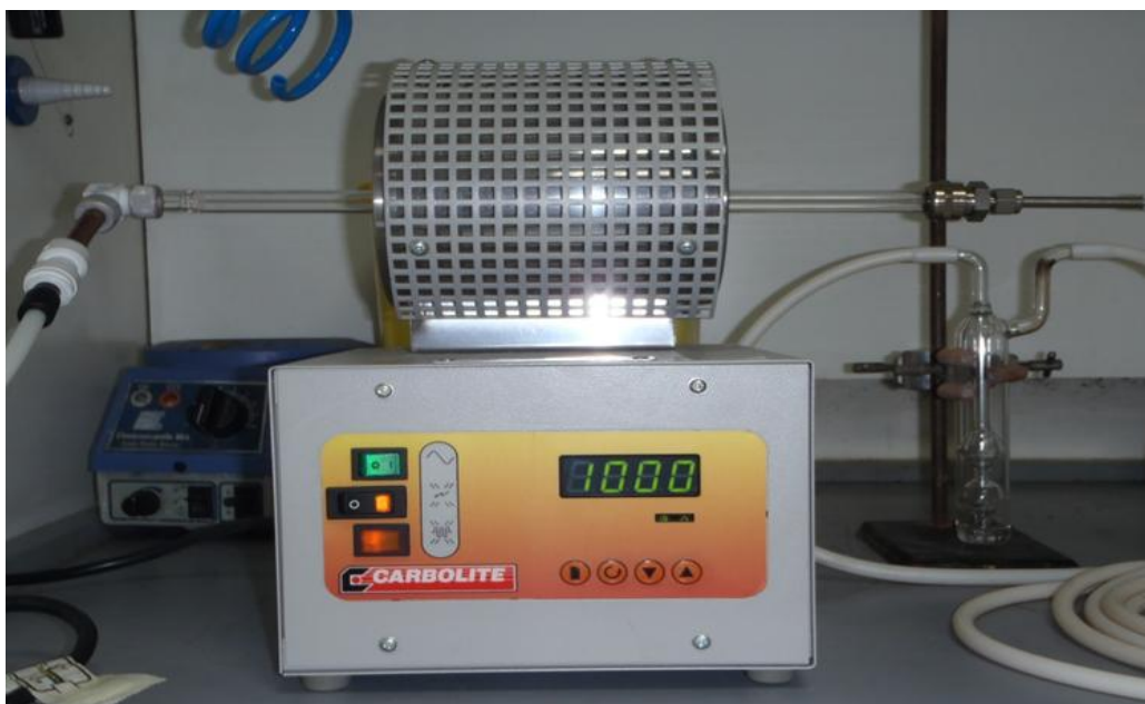
Fig. 3.8: The furnace from the CVD graphene growth system at Durham.
