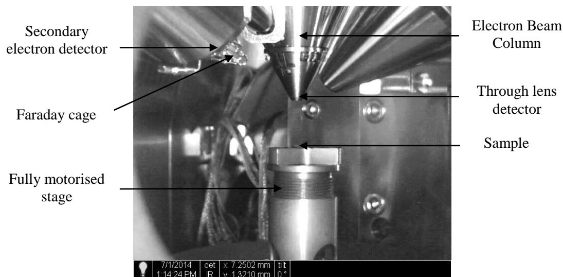
Fig. 3.16: Photograph of the secondary electron detector.
