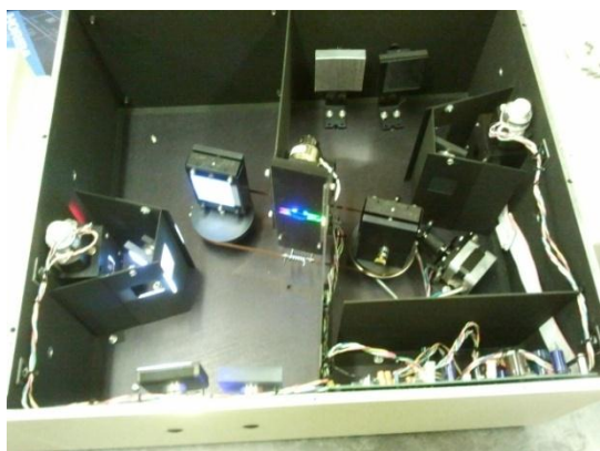
Figure 3-7: (Left) Schematic of the Fluorolog-3 spectrofluorimeter for the collection of photoluminescence and excitation spectra. Light grey lines indicate approximate light paths from source to detector. (Right) Photograph of the inside of the excitation double-monochromator unit, with source lamp excitation arriving from the left of the image.
