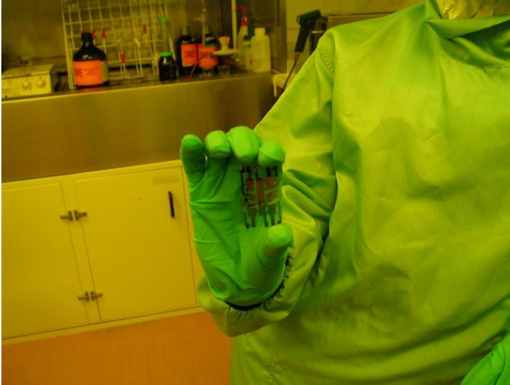
Fig. 3.8. The completed OLED device with 4 big (5 mm x 8 mm) and 4 small (3 mm x 3 mm) pixels.
