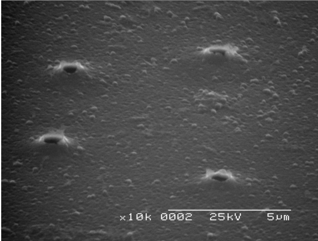
Fig. 4.7. The SEM image of the nanopore device after driving at 21V for several seconds.
