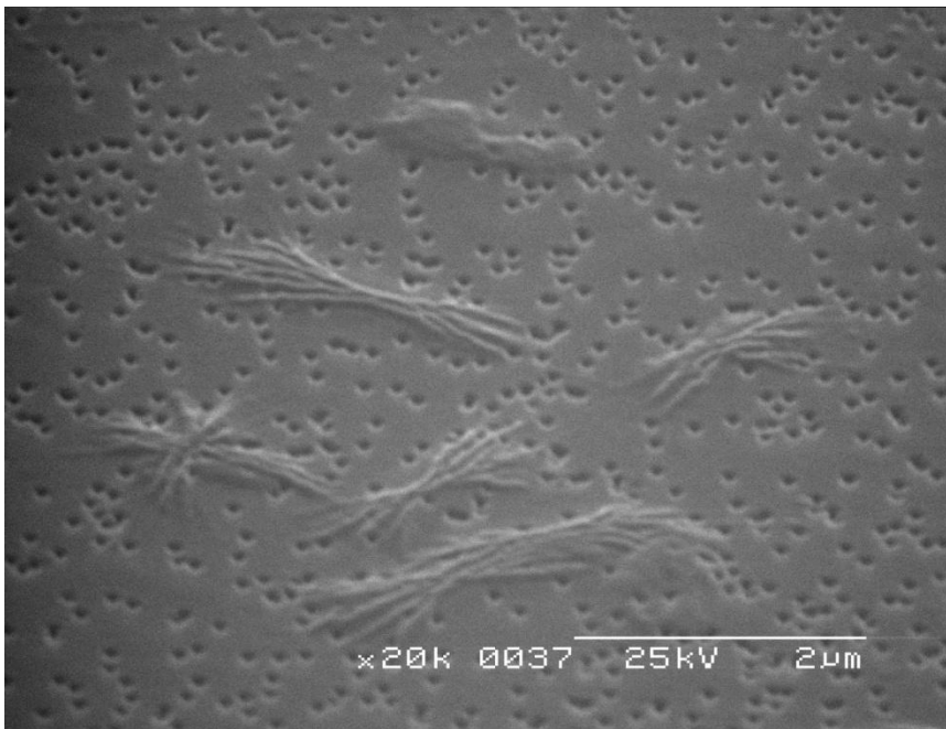
Fig. 4.2. Atomic force microscope (AFM) image (upper) and Scanning electron microscope (SEM) image (lower) for the surface of the nanopore device after all the organic layers are evaporated but before capping the cathode. The diameter of these pores are 110 nm each with a density of 10^9/\text{cm}^2 .
