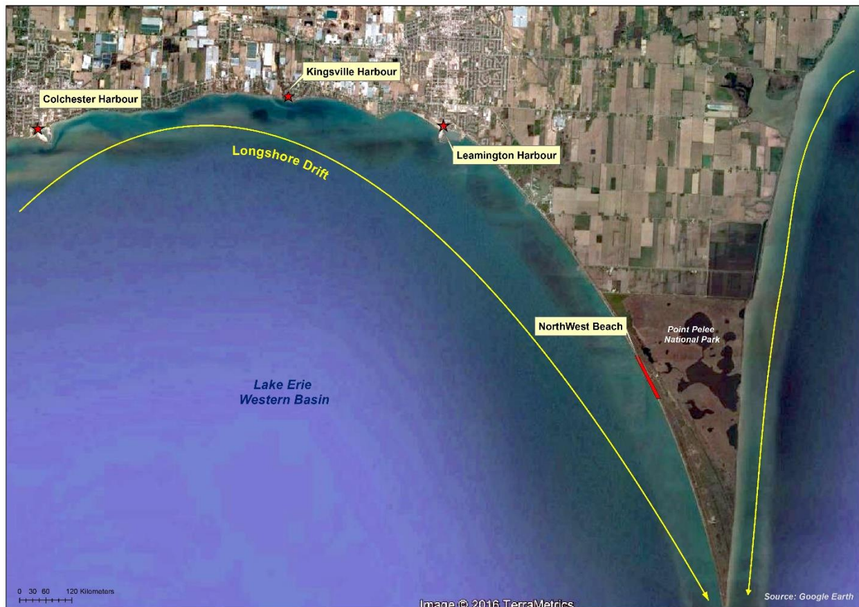
Figure 4.2: 2015 Image showing longshore drift and development of erosional structures along the shoreline (Source: Google Earth image 2015)
