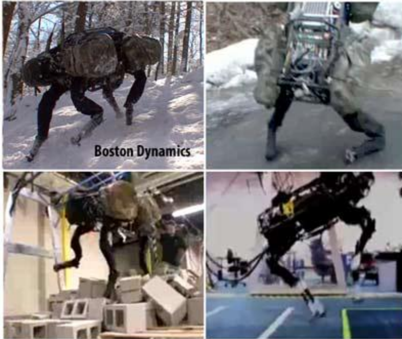
Figure 1.6: Boston Dynamics “Big Dog.” Show here in four different test modes – walking uphill in snow, slipping and recovering balance on an icy surface, climbing an unstable incline, and jumping over an obstacle.
