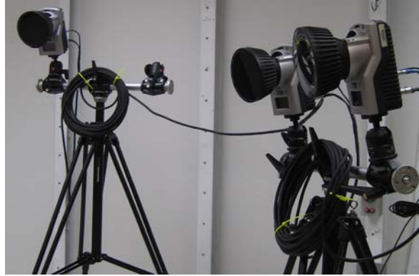
Figure 38. Photograph of the Qualysis 3-camera system used to collect 3-D position data for resolving the specimen's JC.
