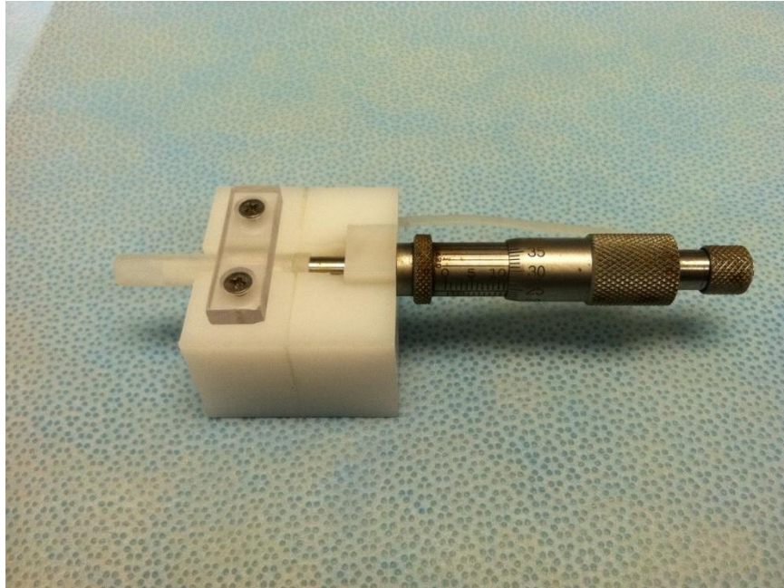
Figure 3.1. Customized cutting device. Device used for separating the Superficial 1/3 and the deep 2/3 of the articular cartilage with accuracy up to 2 \mu\text{m} .
