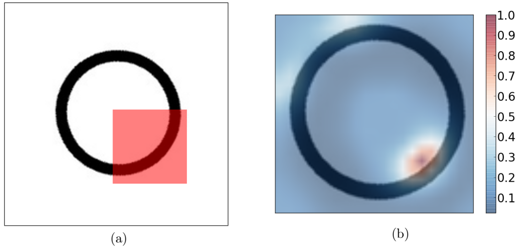
Figure 3.7: (a) Example in which a prototype is "imprinted" from an image, with the selected region shown in red. (b) The S2 activity resulting from applying this prototype to the original image. Red indicates high activity, while blue indicates low activity.
