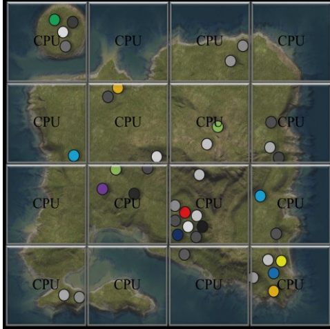
Figure 4: Overhead view of a virtual world using regular grid spatial subdivision. Circles represent entities/players.
