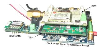
Figure 3.3: Trusted Sensing Peripheral with a Bluetooth and GPS module.
