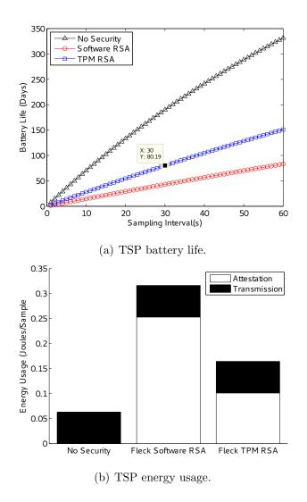
Figure 3.5: Battery life and energy usage of the TSP.
