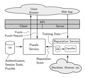
Figure 6.6: Design of MetaCAPTCHA
