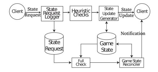
Figure 5.4: Alternative architecture: request validation in parallel
