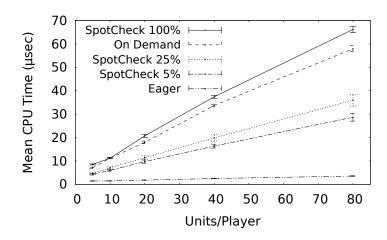
Figure 5.5: Server CPU overhead
