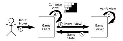
Figure 5.1: After the user enters her move, the game client computes a description of the view (e.g. newly visible map regions). The server trusts the client to compute this view, but occasionally checks if the view descriptor was computed correctly.
