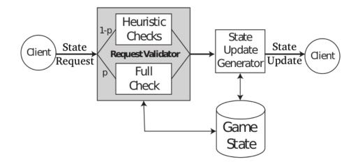
Figure 5.3: SpotCheck server-side architecture
