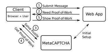
Figure 6.1: System model: user's browser must show proof-of-work before the web application accepts the user's message. The dotted line indicates initial setup performed by the web application to use the MetaCAPTCHA service.
