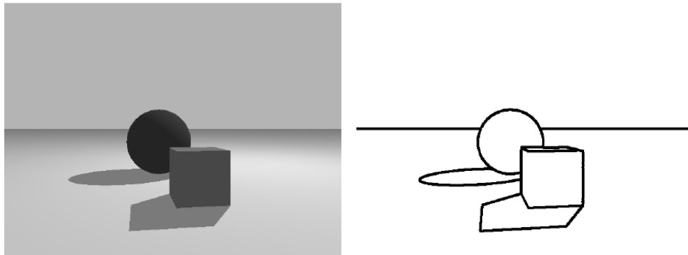
Figure 1.1. Simple, idealized scene of two objects illuminated by a distant point source and homogenous ambient light (left). Discontinuities in the intensity function (right).
