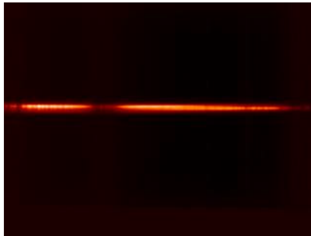
Figure 2-16. A spectral image of the standard star from Figure 14 after being orthogonalized using a quadratic fit for the spatial axis with the refined transformation algorithm.
