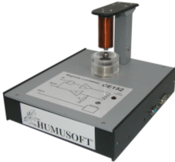
Figure 5.1: CE152 magnetic ball levitation.
