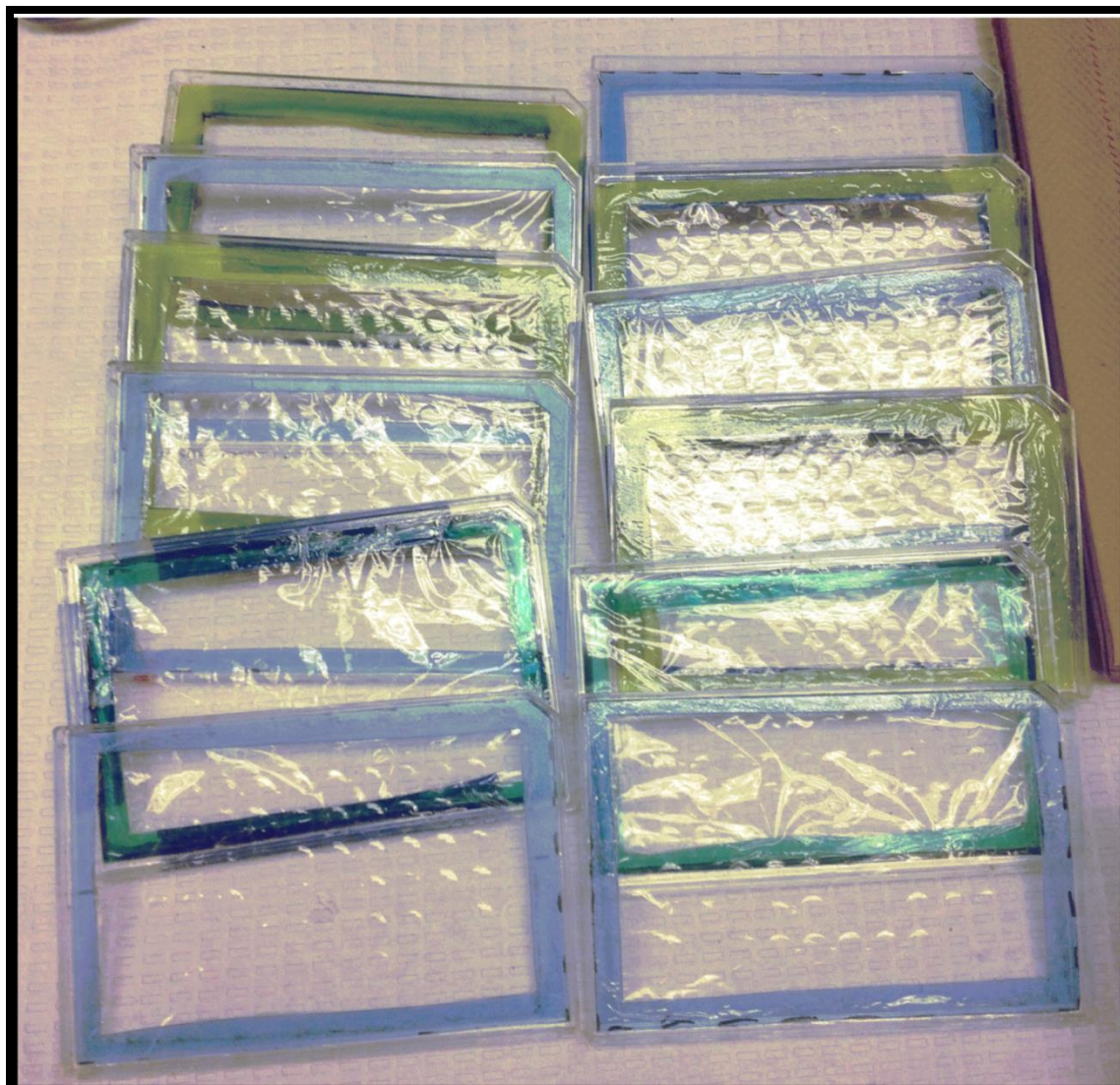
Figure 3.2. Photograph of gasket-attached FEP film lids. The lids were constructed fixing a rectangular gasket (cut from sheets of thick plastic) to a square of FEP film with adhesive. The gasket-film combinations were then glued onto the underside of 96-well plate lids, from which the majority of the top plastic surface had been removed with a hot scalpel. Once placed on top of a microplate, air flow could be completely restricted to the plate, except by passage through the FEP film by, by wrapping the outside edges of the plates with vinyl tape. The durability of FEP film makes it amenable to cleaning by washing with deionized water, and sterilization by cleansing with 70% ethanol. Cleaned plates could then be dried in a sterile environment and reused.
