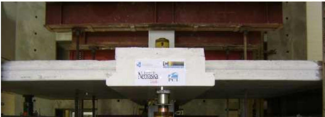
Figure 2.4 – Shallow Hollow-Core Floor System (Tadros and Morcous, 2011)
