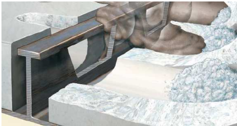
Figure 2.2 – Typical Girder-Slab Floor System (Girder-Slab Technologies, 2008)
