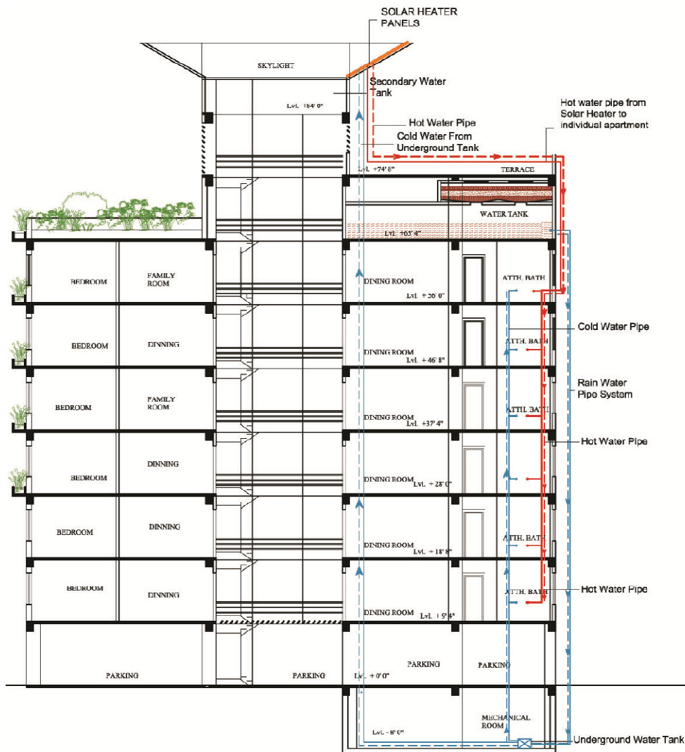
Figure 9.15 - Solar water heating system
