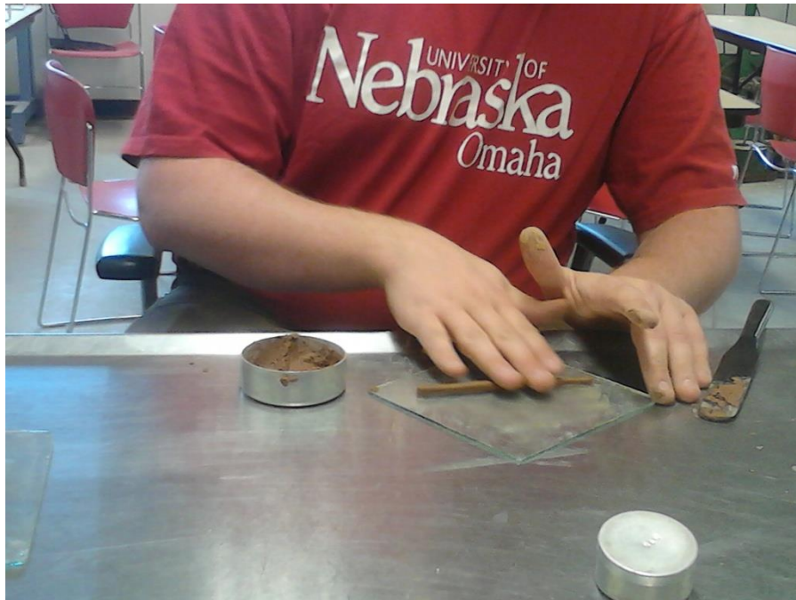
Figure 3.3: Soil molded into threads to determine the Plastic limit Source: Author
