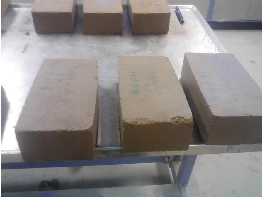
Figure 6.6: Submerged 10% stabilized earth blocks after 24hr
