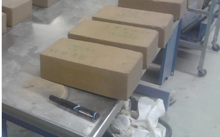
Figure 6.4: 8% stabilized earth blocks after 24hrs submersion
