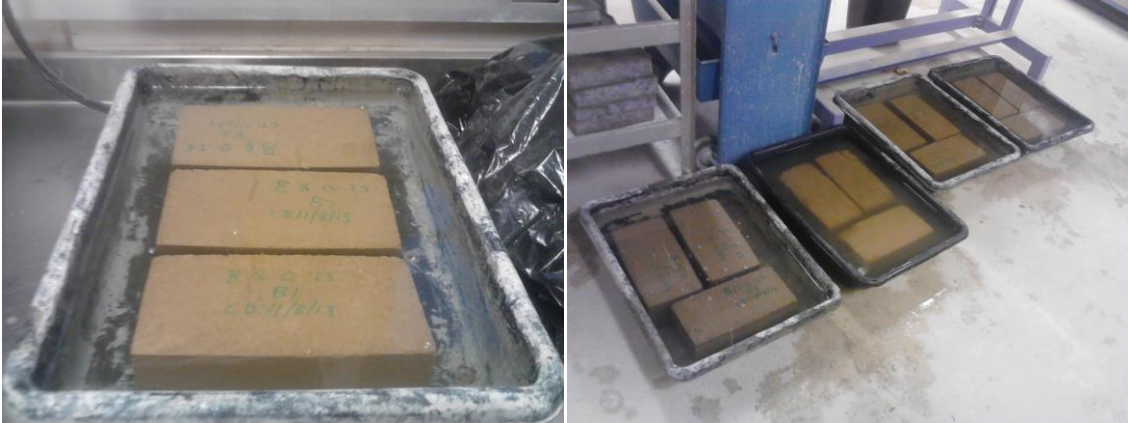
Figure 3.13: Submerged Blocks Source: Author
