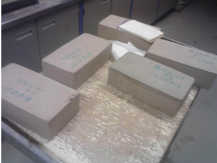
Figure 6.8: Submerged 15% stabilized earth blocks after 24hrs
