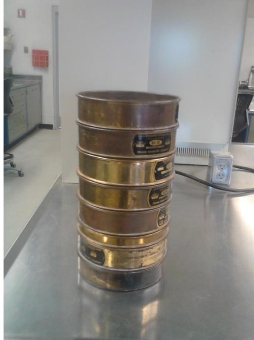
Figure 3.4: Different Sieve pans stack together Source: Author
