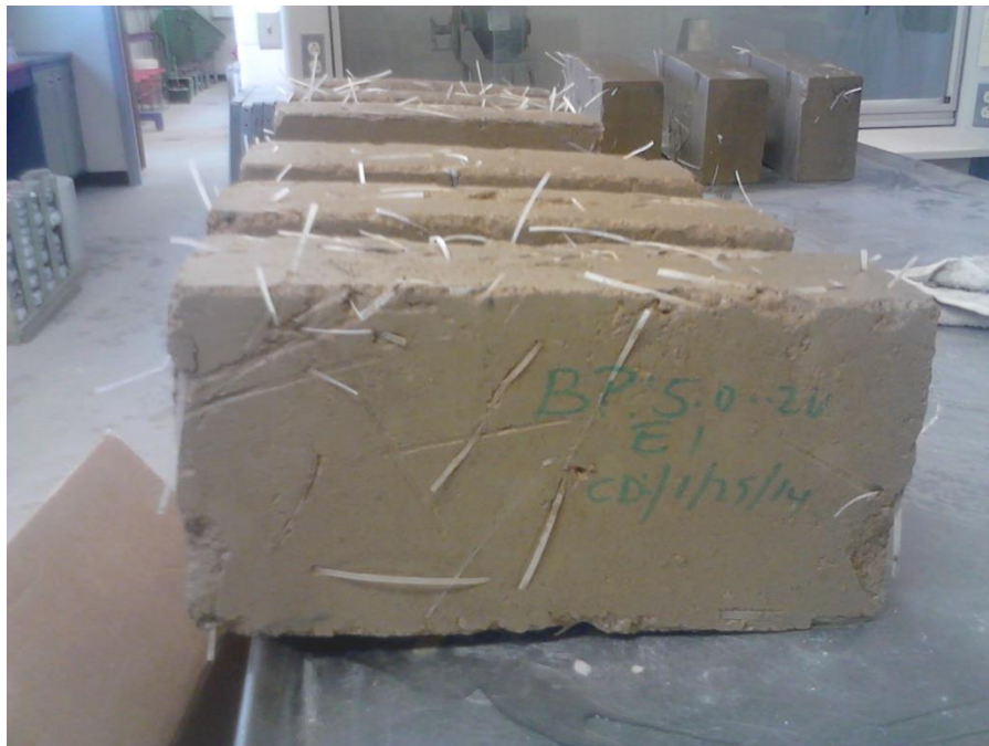
Figure 4.5: 5% stabilized earth blocks after submersion test Source: Author
