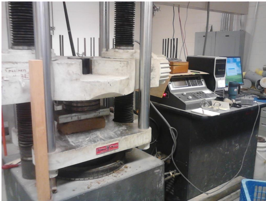
Figure 6.15: Compression test in progress
