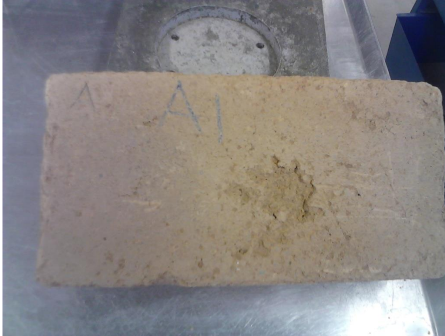
Figure 4.8: Depth of penetration through the blocks Source: Author
