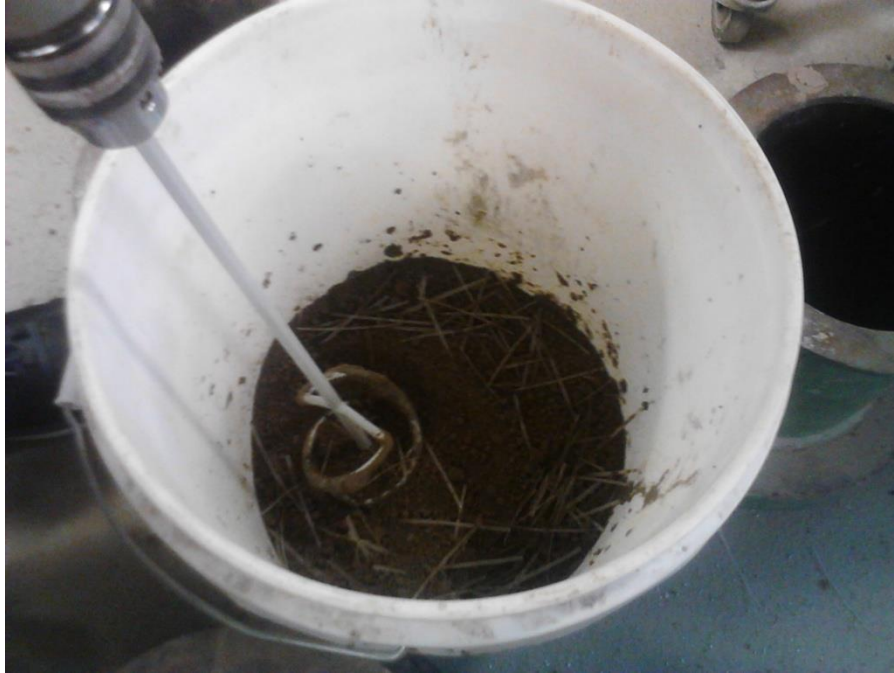
Figure 3.9: Soil, stabilizer, and fibers during the mixing process Source: Author
