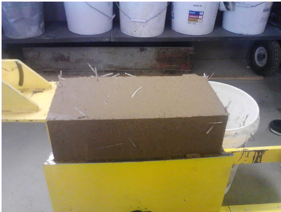
Figure 3.10: Cast Fiber Reinforced CSEB Source: Author
