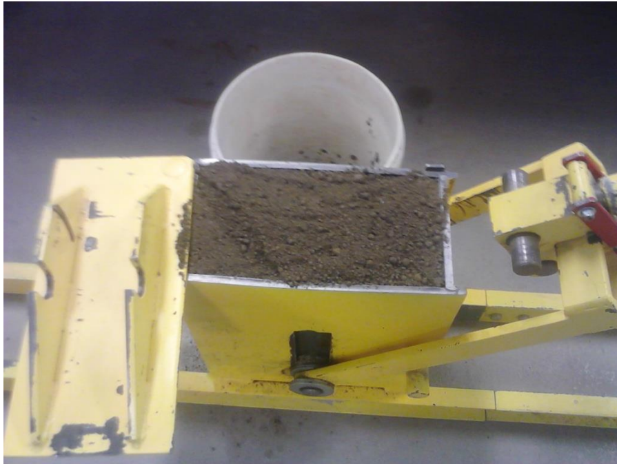
Figure: 3.6: Manual press filled with soil mixture Source: Author
