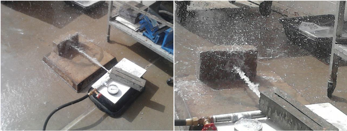
Figure 3.16: Spray test in progress Source: Author
