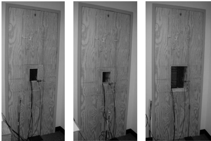
Figure 3.5 – View of aperture and BK2 placement. From left to right, thin/small, deep/small, and deep/large aperture from test room
