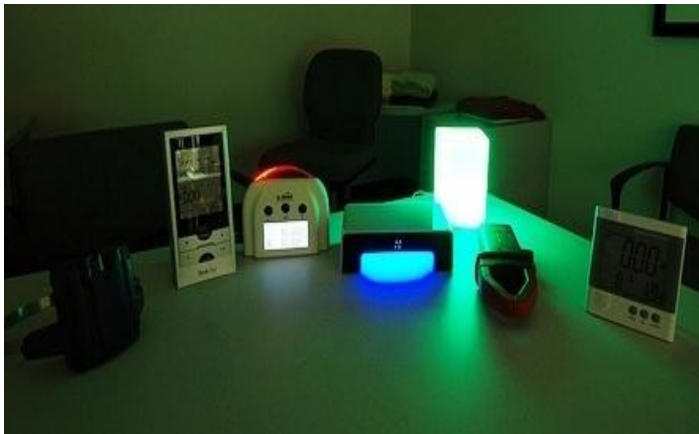
Figure 3: RTM Displays From Left to Right: PCM, Aztech, Wattson, Ambient Orb, Cent-A-Meter [9-10] (photo courtesy of Josh Eiden)
