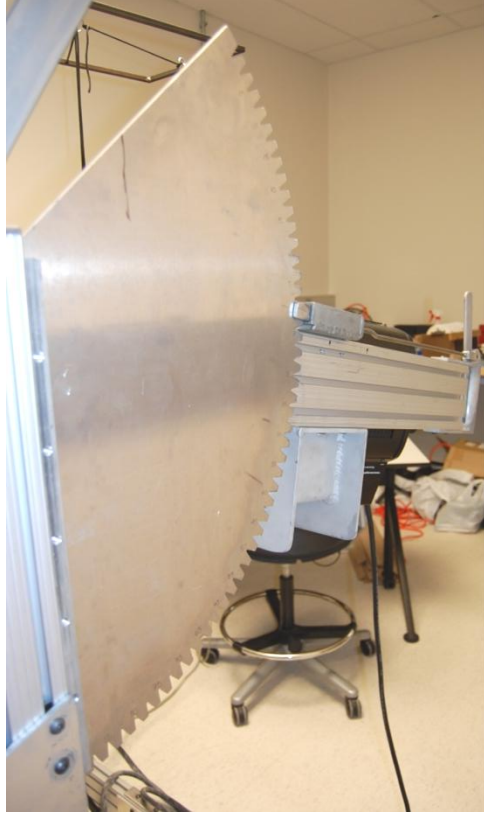
Figure 3-8. Gear used to change the position of the arm
