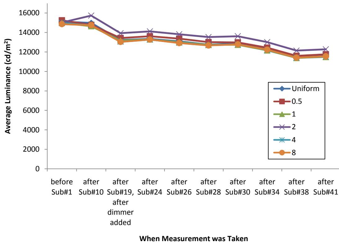
Figure 3-117. Graph of average luminance vs. duration of experiment for paper targets illuminated by left Robert Juliat fixture
