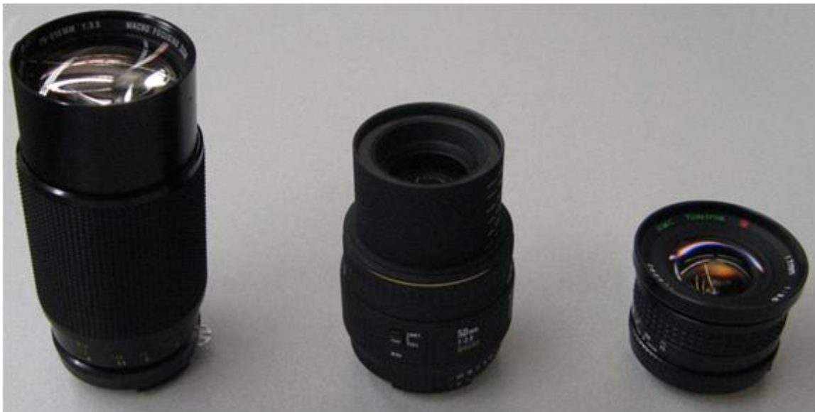
Figure 3-17. Three lenses available for the Digital Imaging Photometer. Lenses are in order from largest to smallest focal length (narrow to wide field of view) from left to right. The focal lengths are 70-210mm, 50mm, and 17mm.
