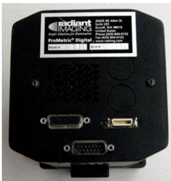
Figure 3-16. View of the back of the digital imaging photometer showing the data connection port (top right) and the power connection port (bottom)
