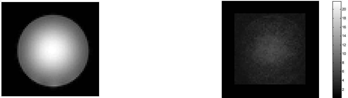
Figure 5.5 Left: EPI phantom image obtained with parameters matched to in vivo data Right: ILC image of EPI phantom plotted on a matched scale
