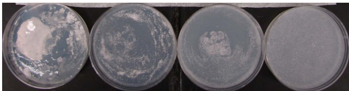
Figure 5-5. Picture of tissue phantoms generated via sonication and vortex mixing. From left to right: TP-1, TP-2, TP-3, and TP-4. Molds are 5 cm in diameter.
