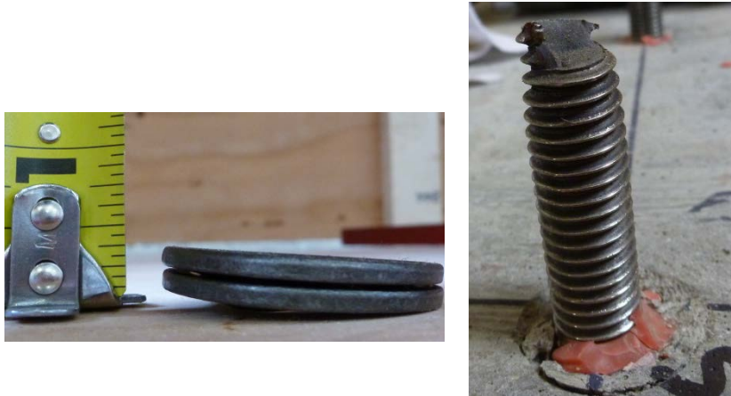
Figure 8.21 Test Series 0b anchor failure and washer deformation
