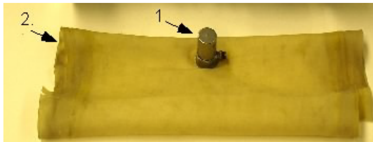
Figure 39: Accelerometer (1) on initial latex membrane (2). (Kalinski, 2012)
