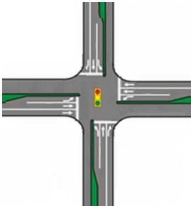
Figure 15: Signalized Intersection (2-Lane Major Street Approach)
