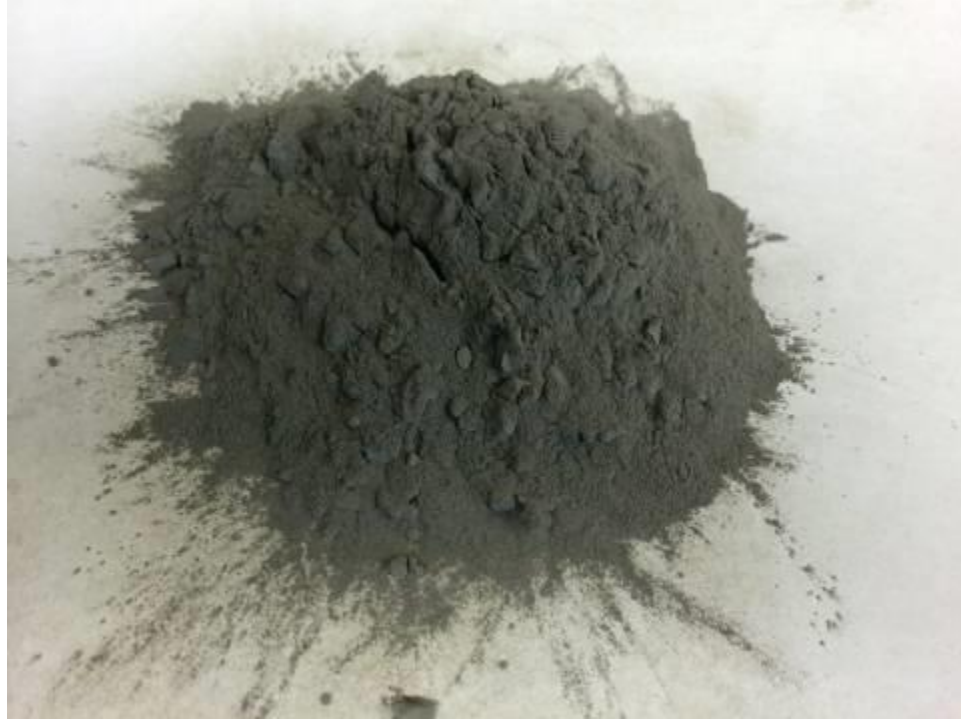
Figure 3.4: Class F Fly ash used in this research
