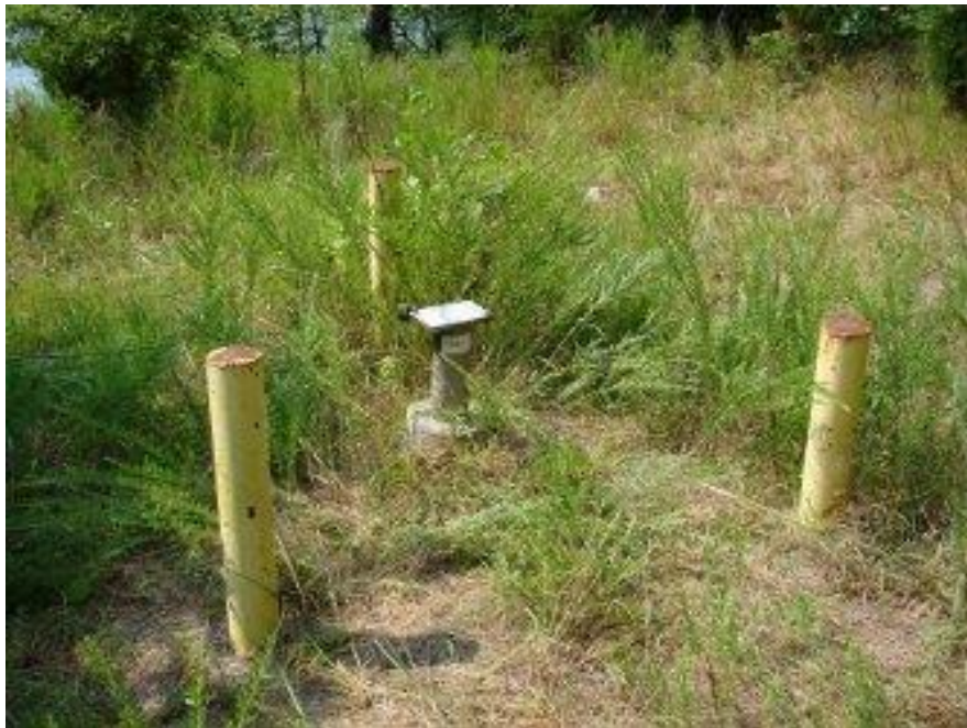
Figure 1.7: Groundwater monitoring well
