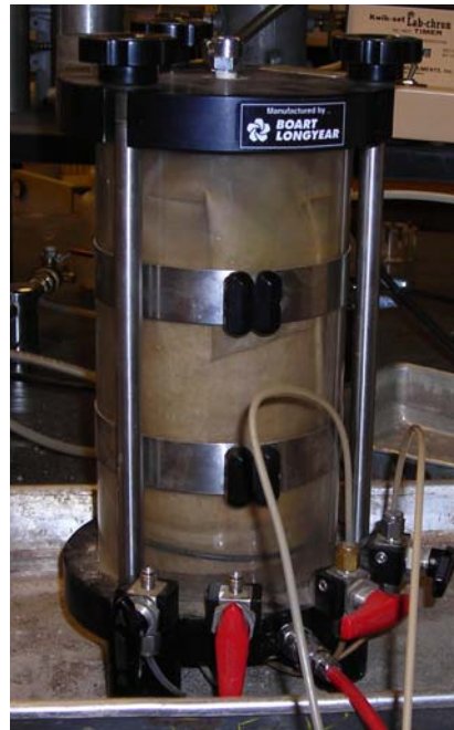
Figure 5.1. Sample setup showing triaxial cell and sample close-up.
