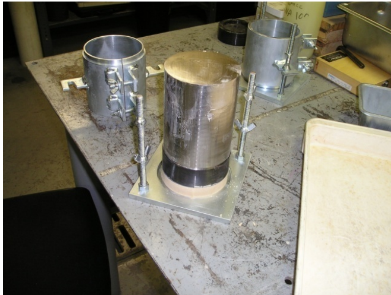
Figure 5.4 – Photograph of the Proctor mold base with gypsum puck, short cylinder, and tall cylinder stacked on top. The cylindrical portion of the Proctor mold had been removed.
