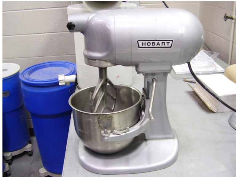
Figure 4.7 – Photograph of the mortar mixer conforming to ASTM C 305 used in the 100% by-product cement project.
