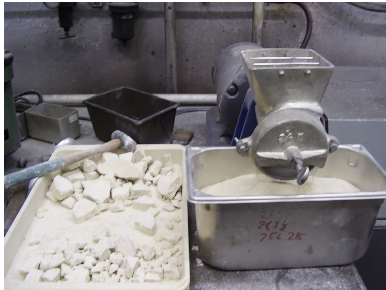
Figure 5.6 – Photograph showing hemihydrate pucks broken up with a hammer and being ground in the disk mill.
