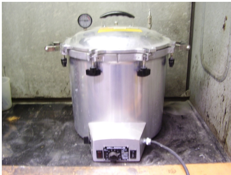
Figure 4.5 – Photograph of the All American Model 75X Pressure Steam Sterilizer used in the production of hemihydrate.
