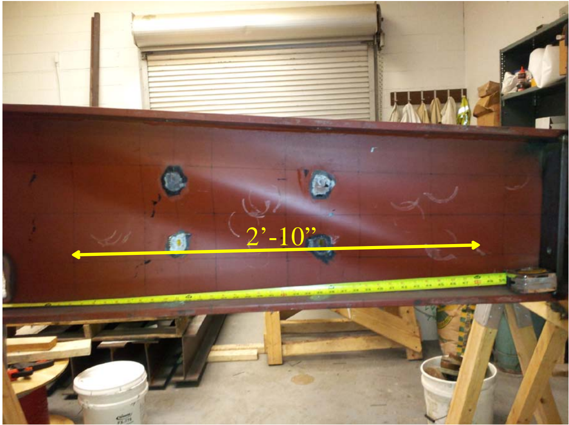
Figure G-1 Web Shear Buckling
