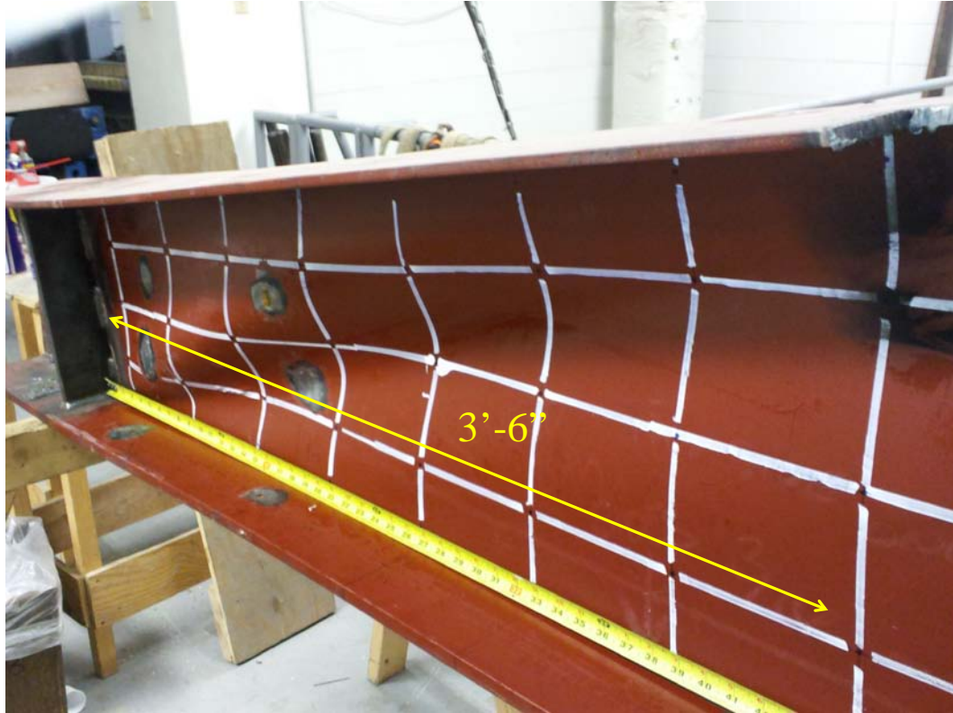
Figure H-1 Web Shear Buckling
