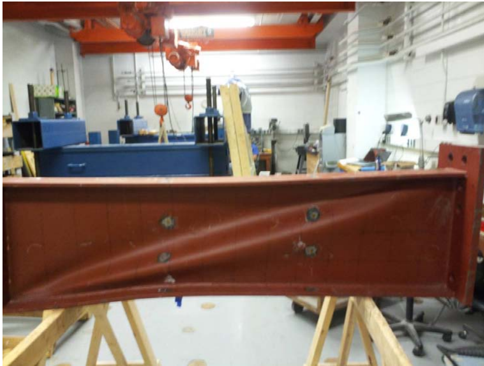
Figure L-1 Web Shear Buckling
