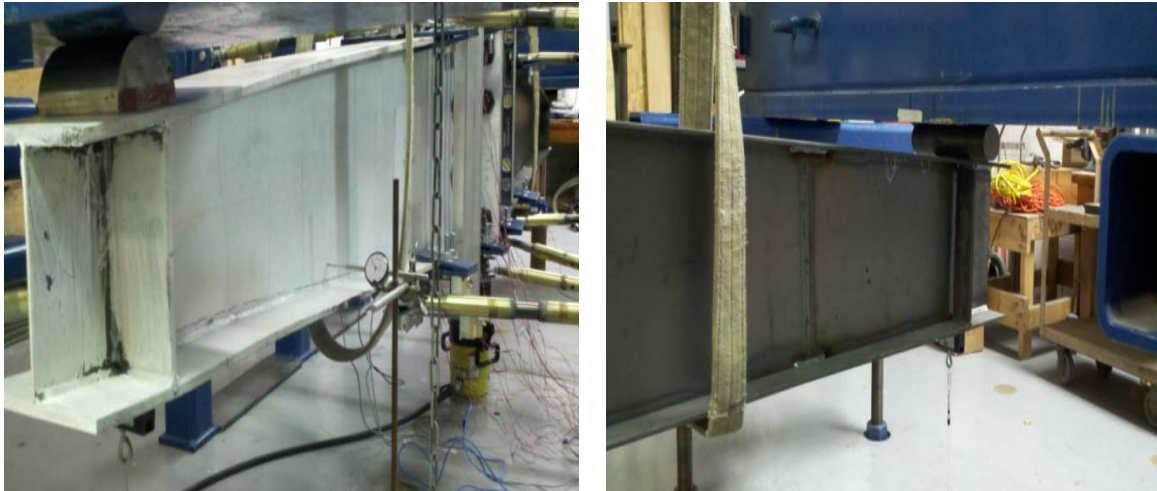
Figure 2-4 Pinned and Roller Supports
