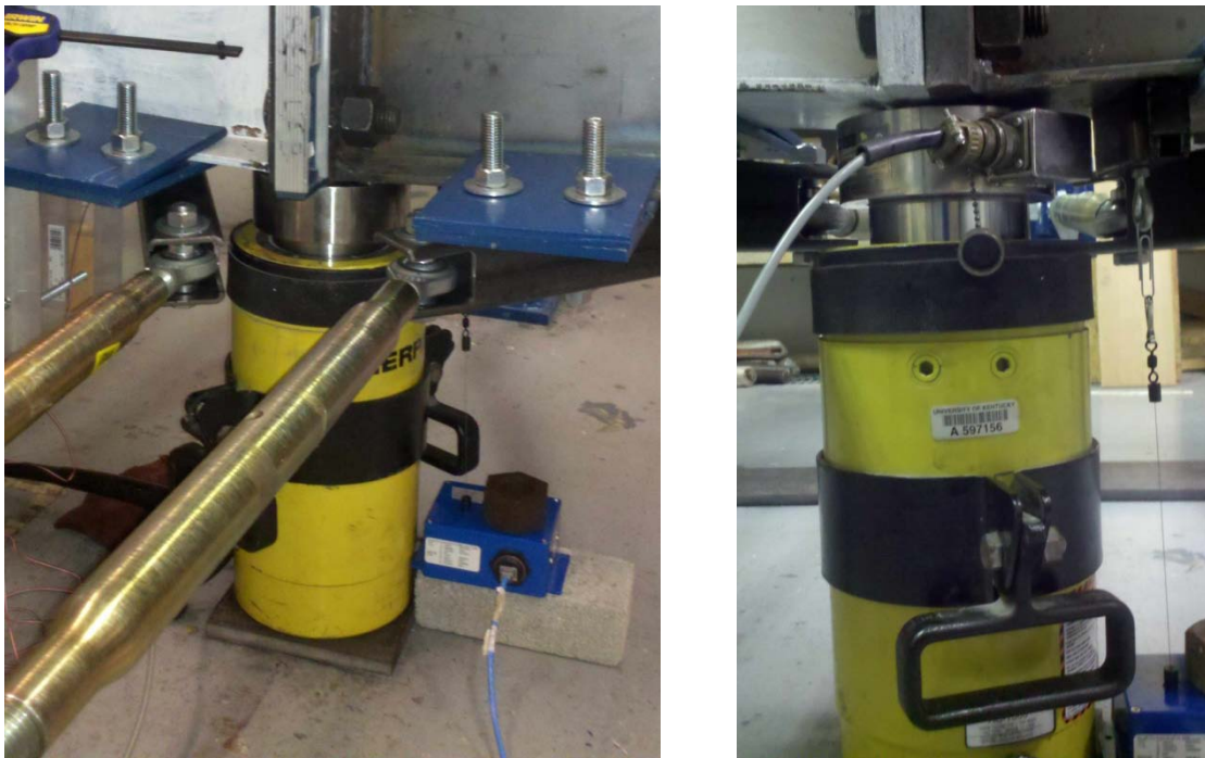
Figure 2-5 Hydraulic Ram and Load Cell
