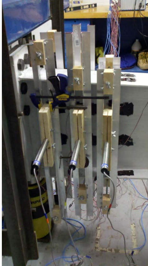
Figure C-1 LVDTs Near Failure Location
