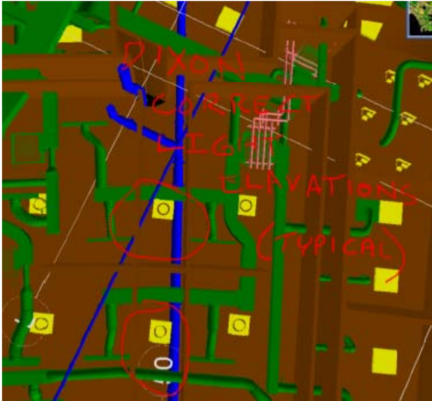
Figure 7.17: Example 4 – Correct Light Elevation
