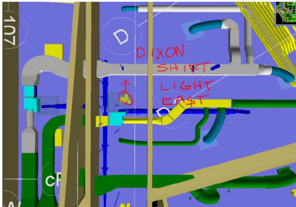
Figure 7.22: Example 9 – Shift Light to Avoid Access Door
