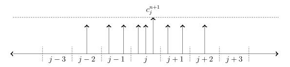
Figure 4.1: Stencil used to advance element j with a three stage Runge-Kutta method on a uniform mesh.
