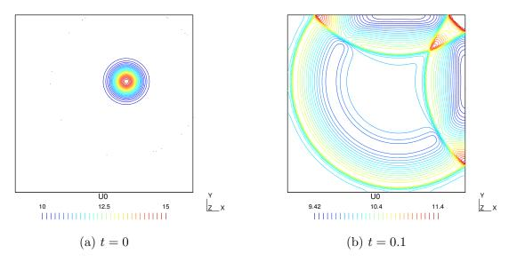
Figure 5.5: Height of the shallow water equations solved using Runge-Kutta 4 local time-stepping.
