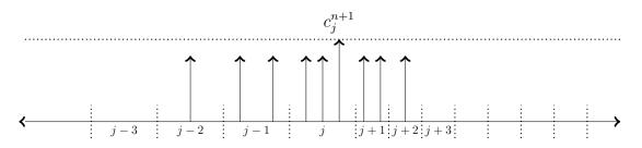
Figure 4.2: Stencil for advancing element j by the local time step size  $\Delta t$  using a three stage Runge-Kutta method on a nonuniform mesh.
