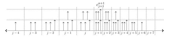
Figure 4.3: Stencil for advancing element j + 1 by the local time step size  $\Delta t/2$  to  $t_{n+1}$  using a three stage Runge-Kutta method on a nonuniform mesh.
