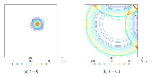
Figure 5.4: Height of the shallow water equations solved using Runge-Kutta 3 local timestepping.
