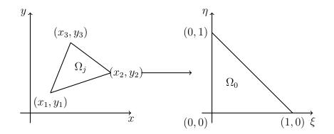
Figure 3.2: Mapping of element  $\Omega_j$  to the canonical element  $\Omega_0$ .
