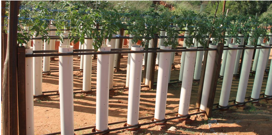
Figure 10.1 Plastic cylinder pipes filled with different soil types and organic matter levels.
