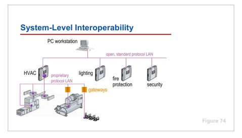
As stated at the beginning of this period, **interoperability** is defined as digital communication between independently manufactured products that are designed to the same open, standard communications protocol. It means that a single controller can monitor and control independently designed microprocessor-based control products.
