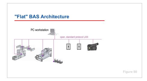
An alternative to tiered architecture uses an open, standard protocol to flatten out the BAS architecture, by connecting the unit-level controllers directly to the main LAN. This approach may reduce hardware costs by eliminating the system-level controllers, but requires the system-coordination logic (scheduling, trending, and optimization routines) to be scattered throughout the network.
