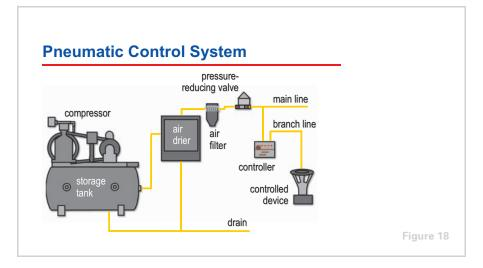
**Pneumatic** control systems vary the pressure of compressed air to operate controlled devices, such as valve and damper actuators. Pneumatic control systems consist of the following major components:
