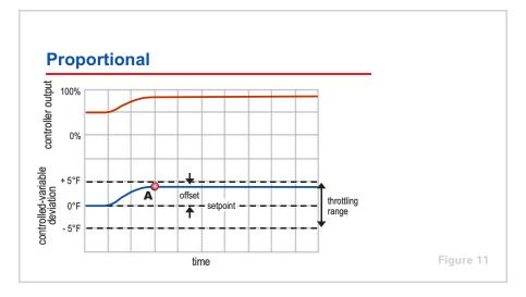
With **proportional** control, the response of the controller is proportional to the deviation of the controlled variable from the setpoint. In other words, the output from the controller is proportional to the difference between the input signal (condition of the controlled variable) and the setpoint.
