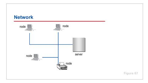
A **network** is the means by which two or more communicating devices are connected together so they can exchange data. Physically, the connections can be made with cables or through a wireless network.
