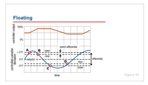
A variation of two-position control is **floating** control, sometimes called three-position control (open-stop-close). Typically, floating control uses a slow-moving actuator and a fast-responding sensor. The controlled device either modulates toward the open position, modulates toward the closed position, or holds its current position.
