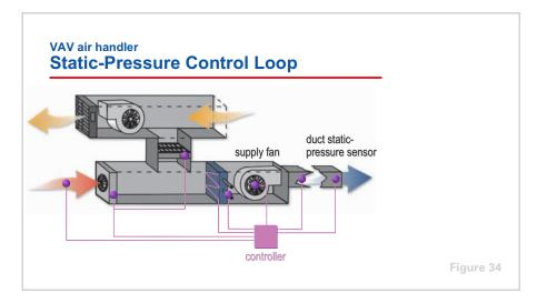
As the cooling load changes, the VAV terminal units vary the airflow supplied to the various spaces served by this system. In response, the capacity of the supply fan in the air handler is modulated to vary the airflow delivered down the supply duct.
