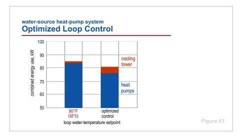
In the example water-source heat pump system, a communicating system-level controller offers the opportunity to optimize the temperature of the water in the loop, minimizing total system energy consumption.
