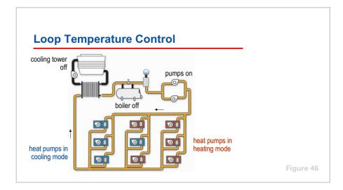
The temperature of the water in the loop is typically controlled between 60°F (16°C) and 90°F (32°C). During warm weather, when all of the heat pumps are operating in cooling mode, heat removed from the air inside the building is transferred to the water loop. This causes the temperature of the water in the loop to increase. A cooling tower, or evaporative water cooler, rejects heat from the water loop to the outdoor air, maintaining a leaving-water temperature of approximately 90°F (32°C).
