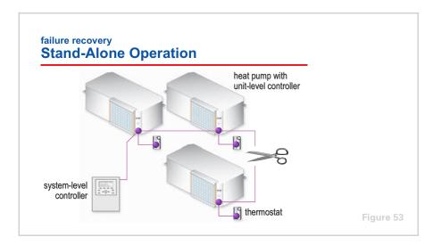
As mentioned earlier, one of the benefits of a distributed control architecture is that it allows stand-alone control of each piece of equipment. In the event that communication with the system-level controller is lost, the unit-level controller should contain a set of instructions and setpoints that would protect the piece of equipment and allow it to continue providing cooling or heating.
