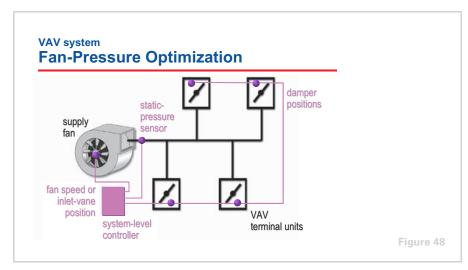
In a VAV system, there is no reason to generate more static pressure in the supply duct than is necessary to push the required amount of air through the most demanding VAV terminal unit. As described earlier, the unit controller on a VAV air handler typically maintains the static pressure in the supply duct. The
