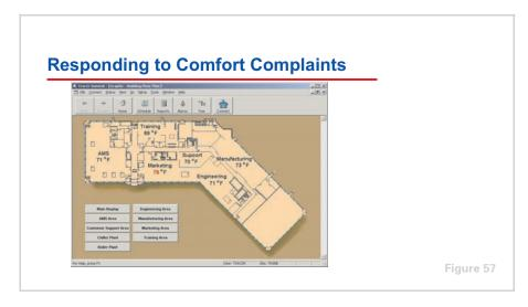
Linking all of the system-level controllers to a building automation system, however, allows the building operator to quickly and efficiently respond to comfort-related complaints from a central location.
