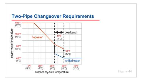
Changing between cooling and heating modes in a two-pipe system requires a lot of excess energy to heat or cool the mass of water in the piping system. Therefore, ASHRAE Standard 90.1–2001 (Section 6.3.2.2.2) includes the following requirements to minimize the energy impact of this switchover:
