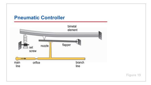
An example of a pneumatic temperature controller is shown in Figure 19. This is a bleed-type controller that uses a nozzle-flapper assembly. A bimetal sensing element, consisting of two different metals fused together, is used to adjust the position of the flapper. As the temperature increases, one metal expands more than the other, and the bimetal element bends in one direction. As the temperature decreases, the element bends in the other direction.
