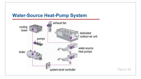
The fourth example system is a water-source heat-pump system. Each heat pump includes a unit-level controller that cycles its compressor to maintain the desired temperature in the zone it serves.
