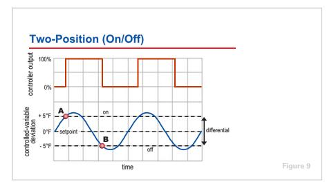
Perhaps the most common control action is **two-position**, or on/off, control. With two-position control, the controller changes the value of the controlled agent from one extreme (open) to the other (closed). This action is taken when the measured condition of the controlled variable goes above or below the setpoint.
