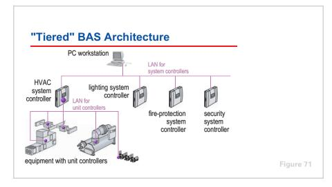
Figure 71 illustrates a conventional approach to installing a building automation system. This tiered architecture delineates subsystems by function. The unit-level controllers on the HVAC equipment are connected to a dedicated network and are coordinated by a separate system-level controller.
