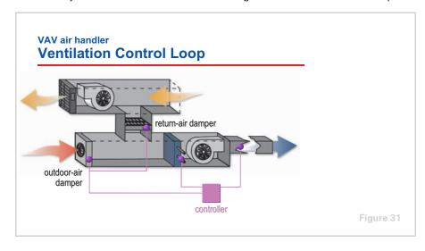
In addition to controlling discharge-air temperature, this example VAV air handler must also ensure that the proper amount of fresh outdoor air is brought into the building for ventilation. In an air handler that delivers a constant volume of air, this typically involves opening the outdoor-air damper to a
