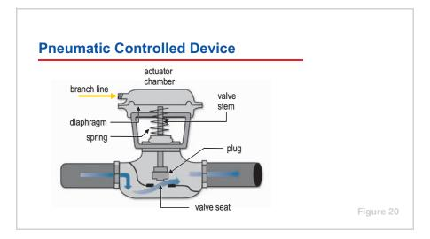
Figure 20 shows an example of a pneumatically-controlled water valve. Compressed air is supplied to the actuator chamber by the branch line. The air pressure in the branch line varies between 3 and 15 psig (21 and 103 kPa). As the compressed air pushes down on the diaphragm, it exerts a downward force on the valve stem. This force causes the plug to move toward the valve seat, reducing the flow of water through the valve.
