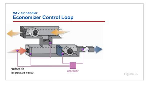
Use of an airside economizer is a common energy-conserving control strategy. It involves using outdoor air as a source of "free" cooling whenever possible. When the outdoor air is cool enough, the air handler switches to the economizer mode and modulates the positions of the outdoor-air and return-air dampers so that the cool outdoor air handles as much of the cooling load as possible.
