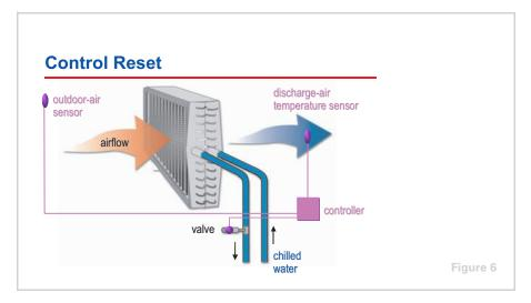
Sometimes, a controller may use a combination of these two loops. In this example, a closed control loop measures the temperature of air leaving the coil, and adjusts the valve to maintain the desired setpoint. A second sensor measures the outdoor temperature. As the temperature of the outdoor air decreases, the controller resets the setpoint to a higher value.
