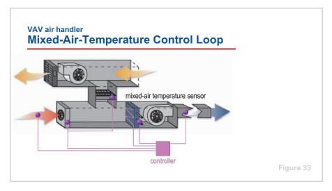
When the dry-bulb temperature of the outdoor air drops below the dischargeair temperature setpoint, continuing to bring in 100 percent outdoor air would require heating the air. At this point, the outdoor-air and return-air dampers modulate, mixing the two airflows to avoid overcooling the mixed air.
