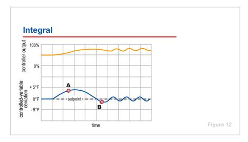
**Integral** control overcomes the offset characteristic of proportional control. It responds based not only on the magnitude of deviation from the setpoint, but also on how long the deviation exists. In response to a deviation from the setpoint, integral control steadily changes the corrective signal sent to the controlled device, returning the controlled variable to the setpoint. It stops adjusting the control signal only after the deviation from the setpoint is zero.
