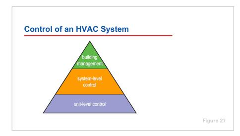
For the purposes of this clinic, automatic control of an HVAC system will be separated into the three levels depicted by the pyramid in Figure 27. The base of the pyramid is formed by the unit-level control of each individual piece of
