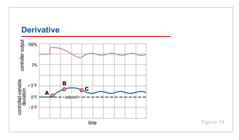
**Derivative** control generates a corrective output signal only when the condition of the controlled variable is changing. When the controlled variable is not changing, the controller takes no corrective action. If the controlled variable is changing quickly, the corrective action of the controller is more dramatic.
