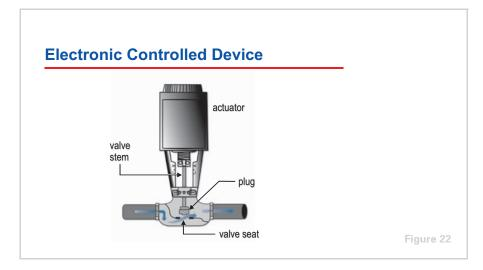
Similar to the pneumatically-controlled valve, the body of a valve used in an analog-electric control system also contains a plug that travels up and down to vary the flow of water through the valve. The difference is in the valve actuator.
