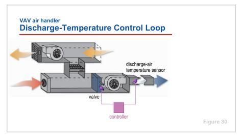
Unit-level control for a piece of HVAC equipment typically involves the use of several control loops. To demonstrate this, assume that the same example cooling coil that was introduced in Period One is installed inside a variable-air-volume (VAV) air handler. This air handler delivers a variable quantity of constant-temperature air down the supply-duct system.
