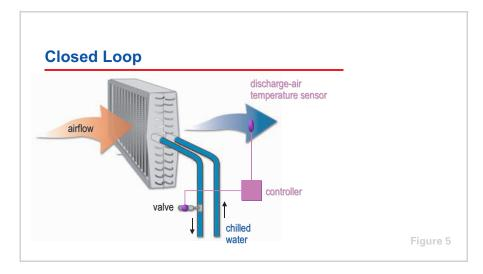
The **closed loop** strategy senses the actual condition of the controlled variable. In this example, the controller compares the temperature of the air leaving the coil to the desired setpoint, and adjusts the valve to meet that desired temperature. In other words, closed-loop control is based directly on the condition of the controlled variable, such as the leaving-air temperature in this example.
