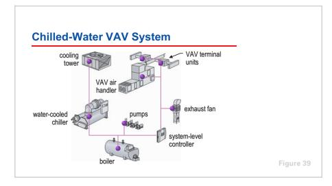
The first example system uses the same VAV air handler that was introduced earlier in this period. This air handler is equipped with a unit-level controller, as are each of the VAV terminal units to which the air handler delivers air. The water chiller that provides cold water to the cooling coil, and the boiler that provides hot water to the heating coils, also have their own, individual, unit-level controllers.
