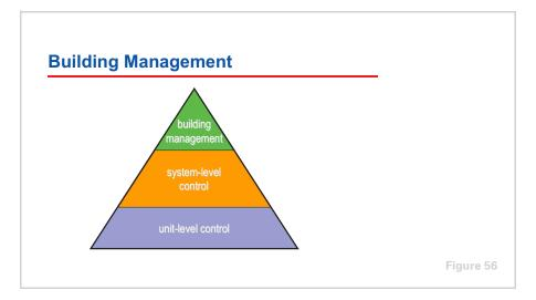
The building-management level is the top level of the pyramid. The hardware needed for this top level is typically a personal computer (PC) with communications ports, a color display, and a printer.
