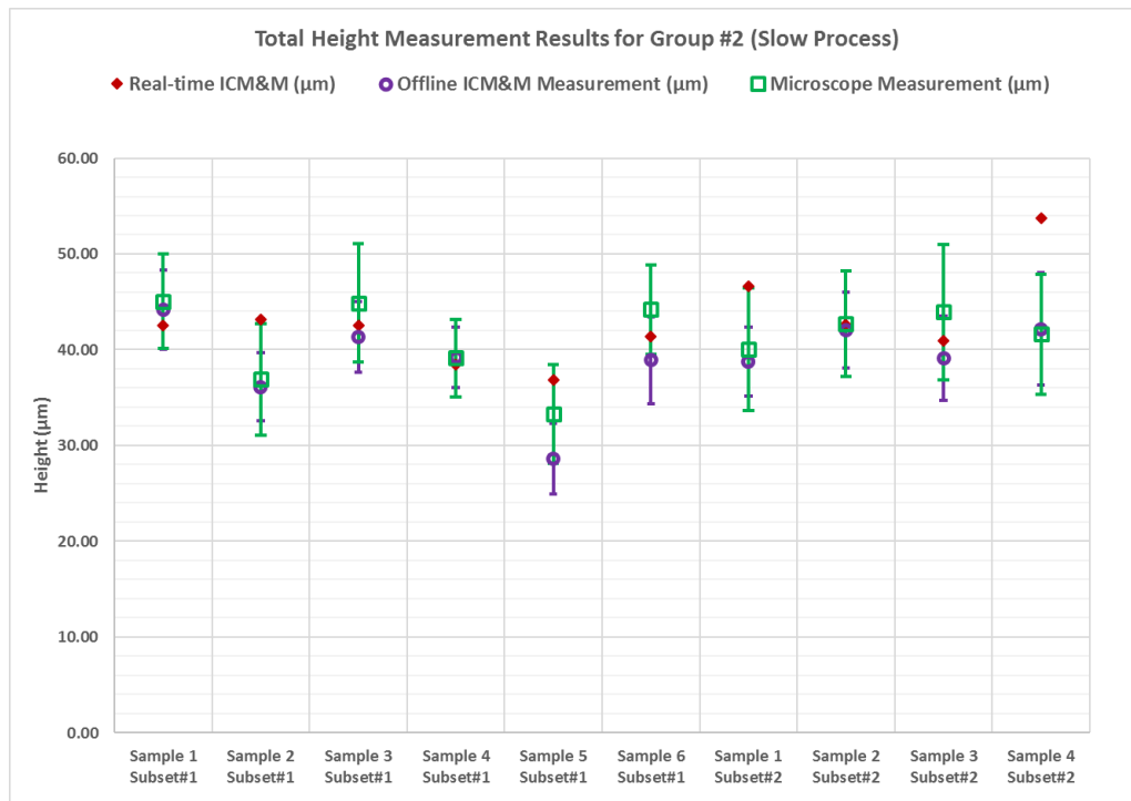
Figure 83. Measurement results of total height for the parts cured in the real-time measurement and control experiments Group #2
