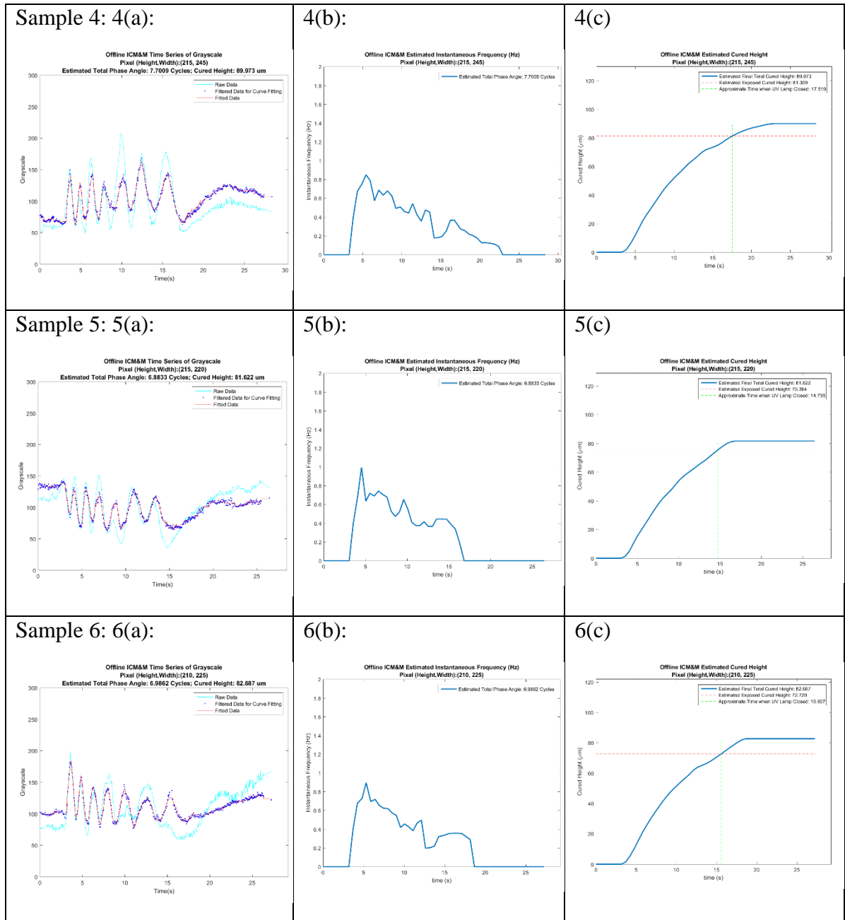
Figure A7 (Part 2). Example of individual pixel's data dynamics and measurement results in the offline ICM&M analysis (Real-time Group #1): (a) time sequence of pixel's grayscale and data analysis; (b) estimated evolution of the instantaneous frequency; (c) estimated time curve of cured height.
